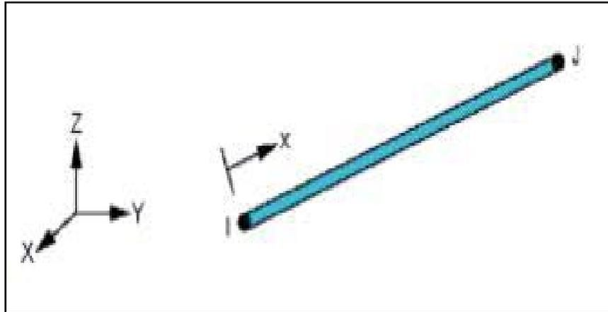
Fig. (9): LINK8 geometry [14]
