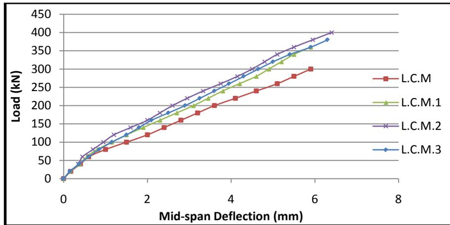
Fig. (6): Experimental load versus mid-span deflection curves
