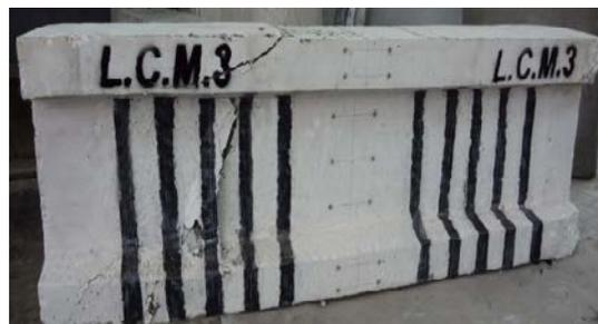
**Fig(5): Shear cracks pattern of L.C.M.3 beam.**
