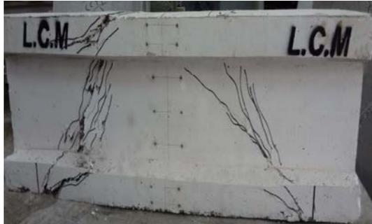
**Fig. (2): Shear cracks pattern of L.C.M beam.**
