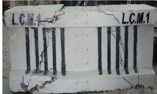
**Fig(3): Shear cracks pattern of L.C.M.1 beam.**
