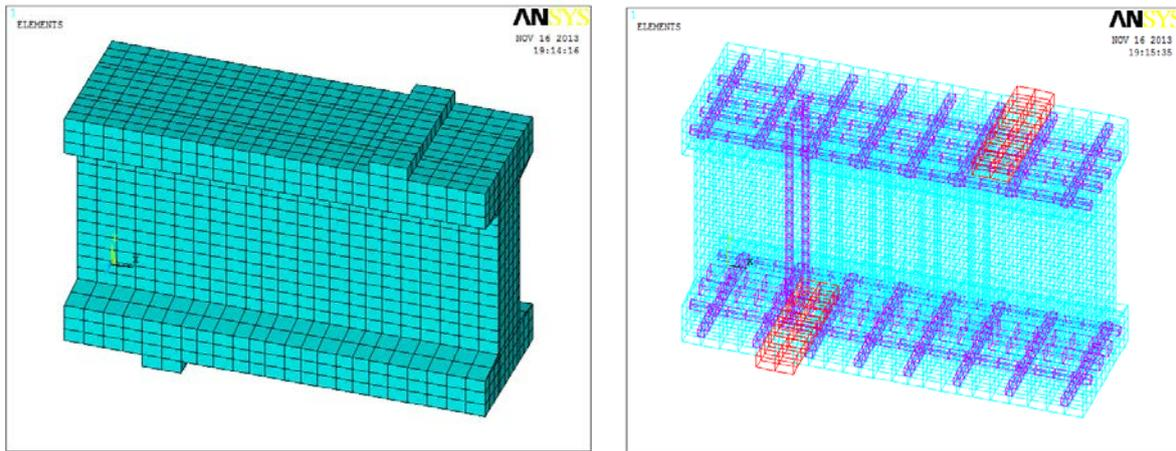
Fig. (11): Typical half symmetry finite element model
