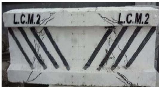
**Fig. (4): Shear cracks pattern of L.C.M.2 beam.**
