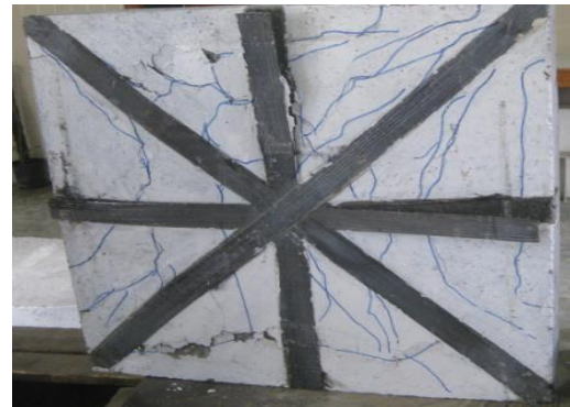
Figure7:Behavior of slab under loading & Crack
