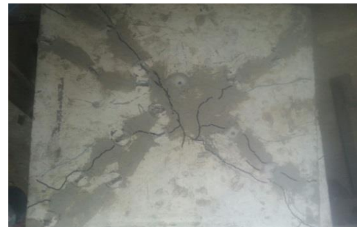
Figure 4.4 : Slab (S6) after repairing and retesting
