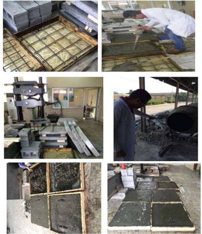
Figure 1: The steps of casting process
