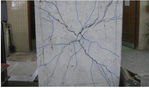
Figure 4.5 : Slab (S11) after repairing and retesting
