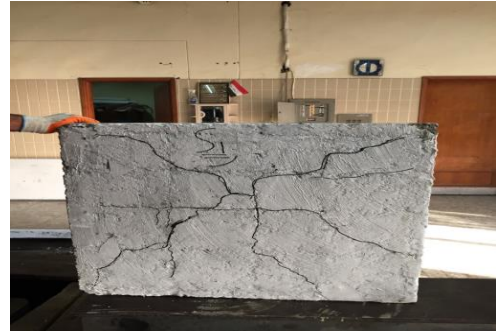
Figure 4.1: Slab (S1) after repairing and retesting
