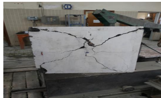
Figure 4.3 : Slab (S4) after repairing and retesting
