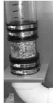
Figure 2: constructed device for permeability test.
