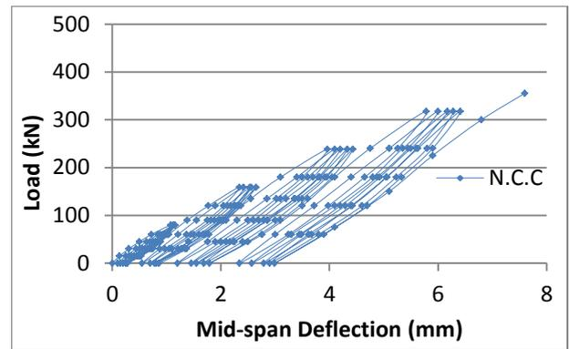
Figure 8: Experimental load versus mid-span deflection curve for N.C.C
