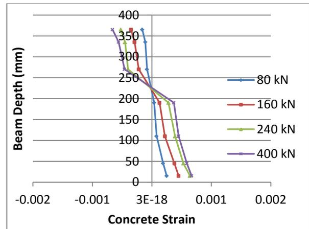
Figure 14: Concrete strain distribution for deep beam N.C.M.2
