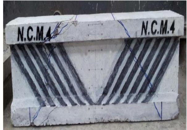
Figure 6: Shear crack patterns of N.C.M.4 beam.
