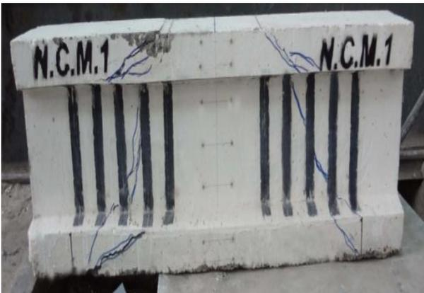
Figure 3: Shear crack patterns of N.C.M.1 beam.
