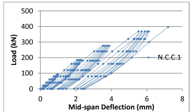
Figure 9: Experimental load versus mid-span deflection curve for N.C.C.1
