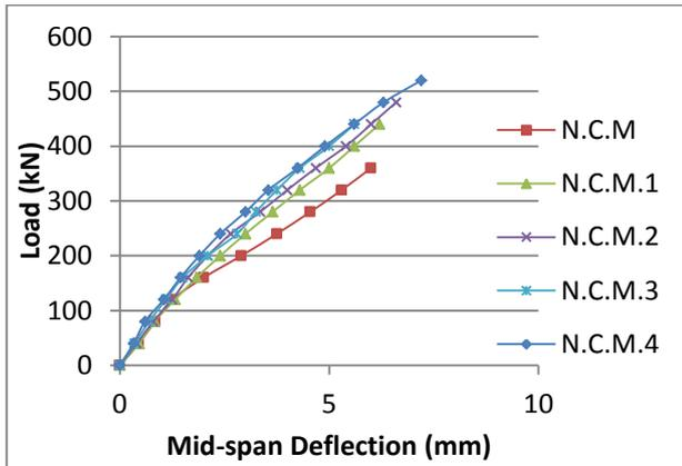
Figure 7: Experimental load versus mid-span deflection curves for the first group
