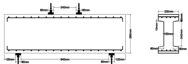
**Figure 1: Reference deep beam (control beam).**
