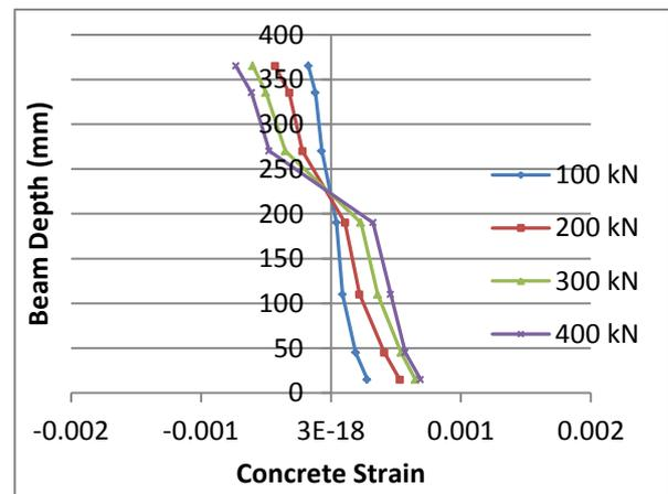
Figure 16: Concrete strain distribution for deep beam N.C.M.4
