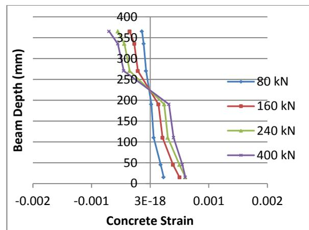
Figure 15: Concrete strain distribution for deep beam N.C.M.3
