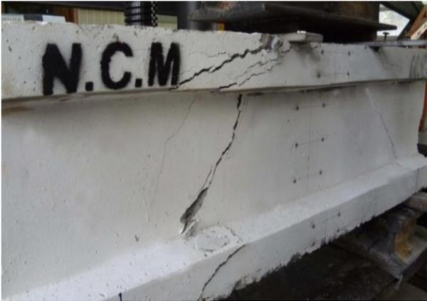
Figure 2: Shear crack patterns of N.C.M beam.
