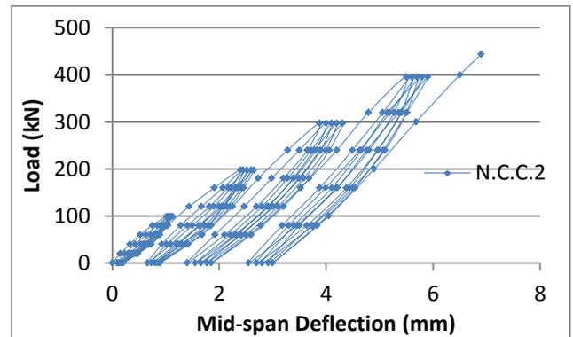
Figure 10: Experimental load versus mid-span deflection curve for N.C.C.2
