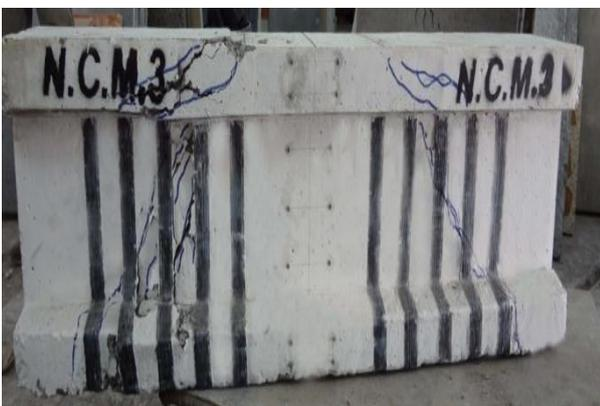
Figure 5: Shear crack patterns of N.C.M.3 beam
