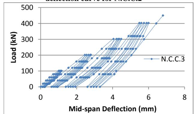
Figure 11: Experimental load versus mid-span deflection curve for N.C.C.3
