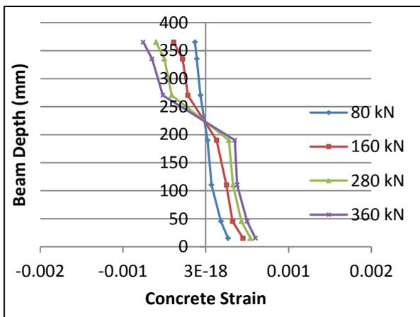
Figure 13: Concrete strain distribution for deep beam N.C.M.1
