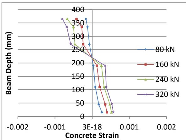
Figure 12: Concrete strain distribution for deep beam N.C.M
