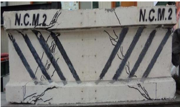
Figure 4: Shear crack patterns of N.C.M.2 beam.
