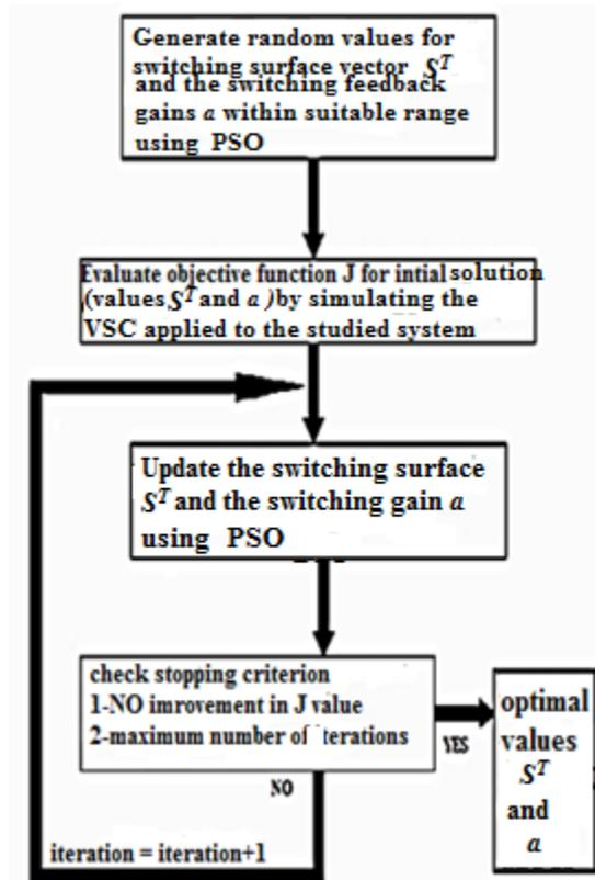
Figure.7: Flowchart of optimal VSC
