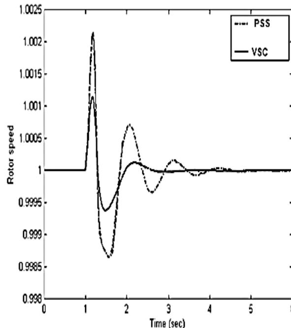
**Figure 11: Response of generator rotor speed at light loading**
