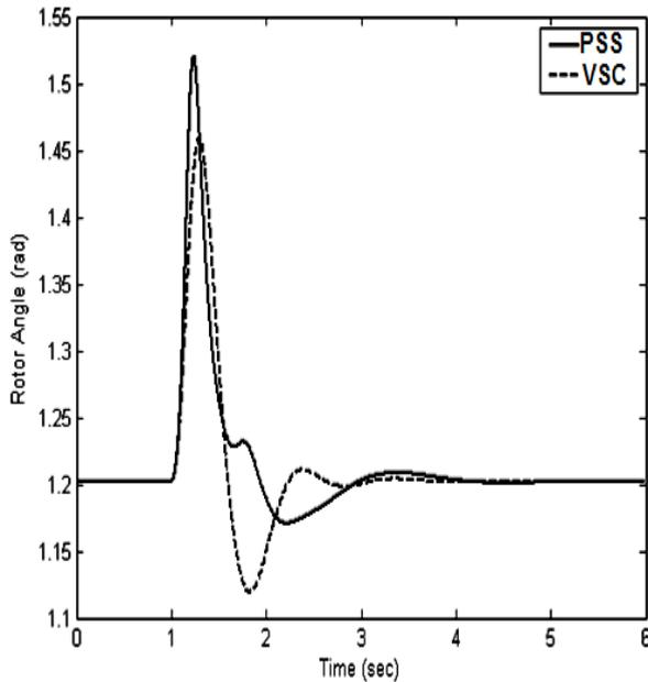
**Fig 8: Response of generator rotor angle at nominal loading**
