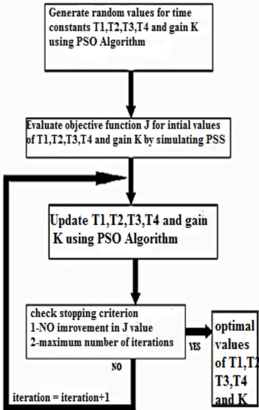
Figure 6: Flowchart of optimal PSS
