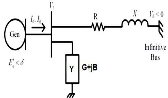
**Figure 1: single machine infinite bus system**
