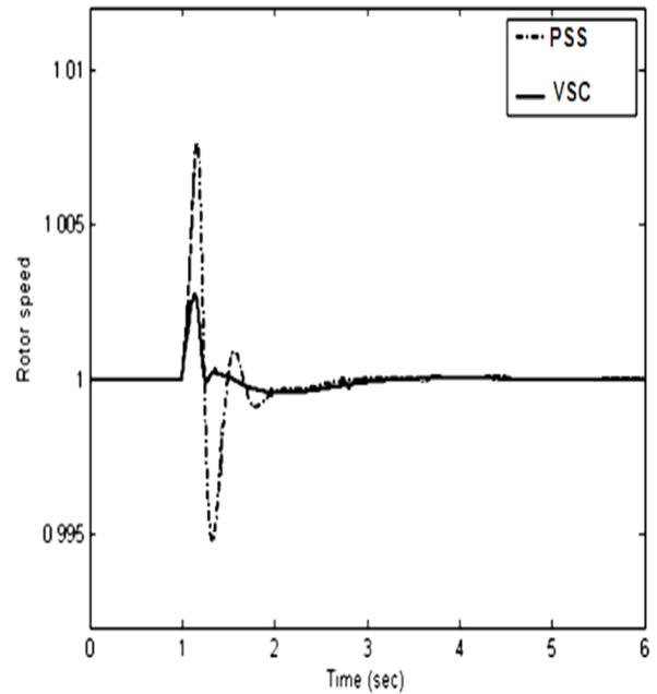
**Figure 9: Response of generator rotor speed at nominal loading**
