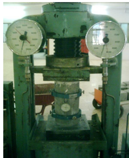
Figure 2: Machine used for compression test and the heat sensor used for taking
