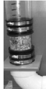
Figure 2: constructed device for permeability test.
