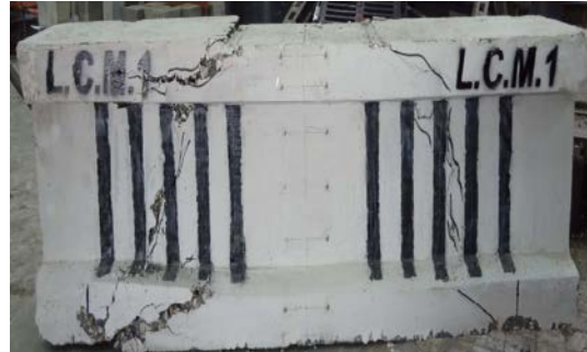
Fig(3): Shear cracks pattern of L.C.M.1 beam.
