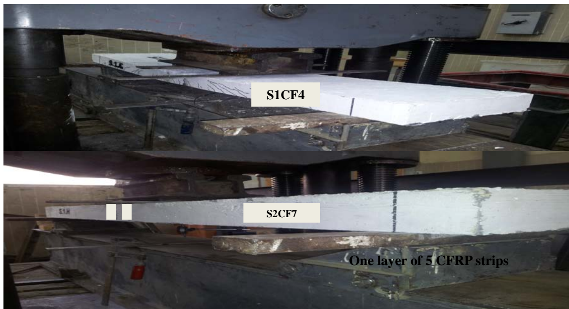
Fig. (5): Picture of the slabs in the testing machine
