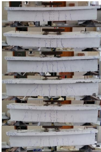
Figure 2. crack pattern for the T-beams failed in flexure
