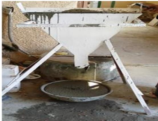
Figure 2: V-funnel test
