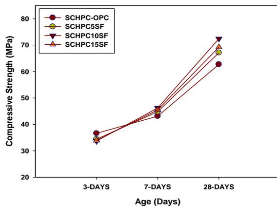
**Figure 5: Compressive strength development of SCHPC containing silica fume with respect to age**
