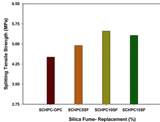
**Figure 6: Influence of SCHPC mixtures containing silica fume on splitting tensile strength at 28-days curing.**
