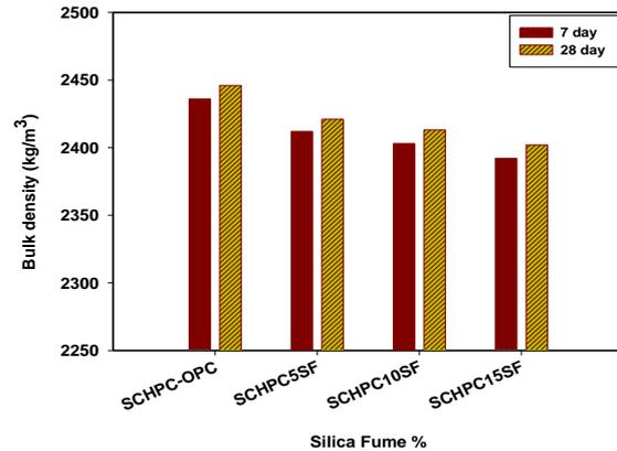
Figure 4: Bulk density of SCHPC containing silica fume with age
