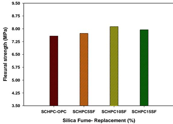
Figure 7: Flexural strength of SCHPC mixtures containing silica fume at 28-days curing.
