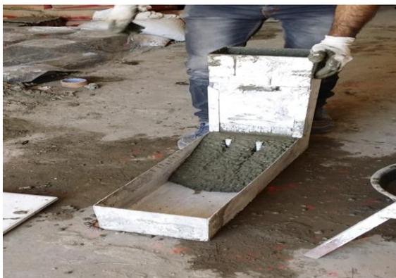
Figure 3: L-box test
