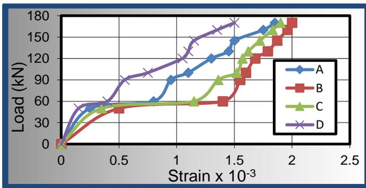
Figure (11): Concrete load- strain curve for (BM25) beam
