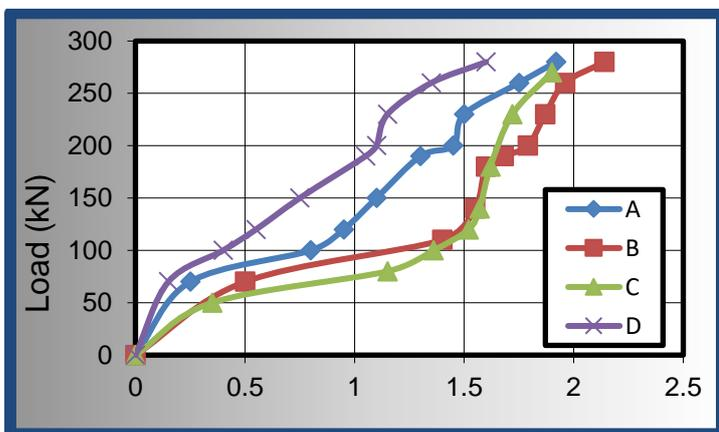
Figure (12): Concrete load- strain curve for (BM30) beam
