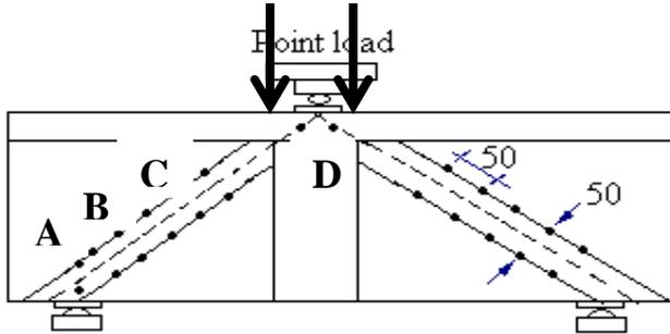
Figure (10): Locations of demec point in test beams
