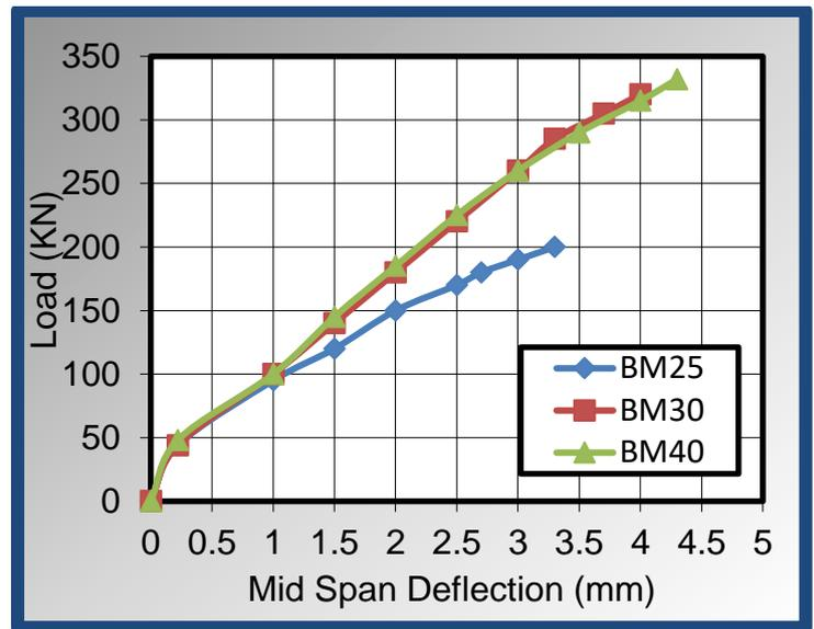
**Figure (8): Experimental load versus mid- span deflection curve**
