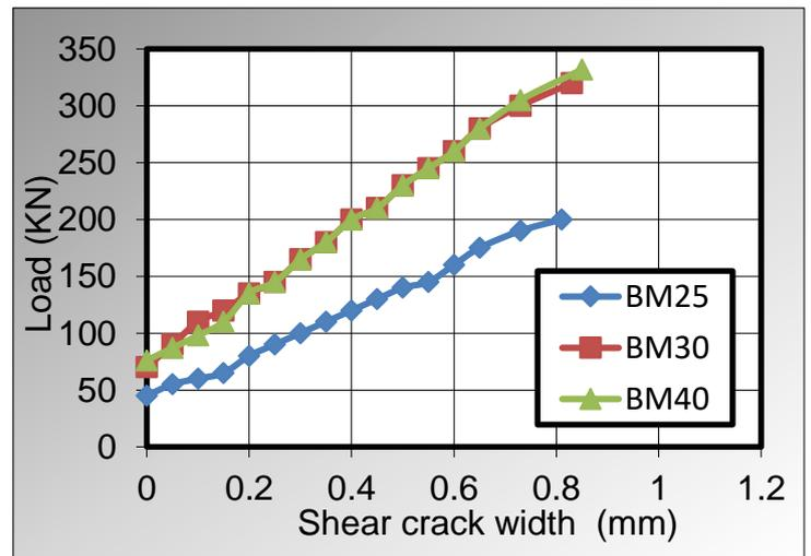
**Figure (9): Load versus crack width of deep beams**
