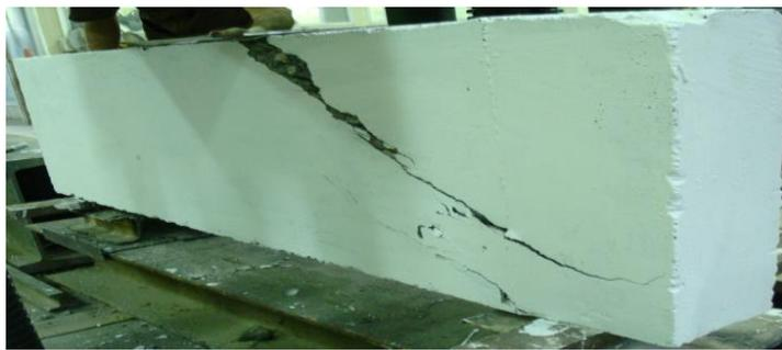
**Figure(7) Shear crack pattern after testing deep beam**
