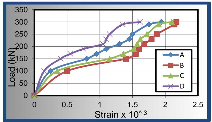
Figure (13): Concrete load- strain curve for (BM40) beam
