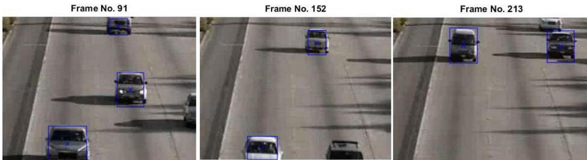
Figure 7: Example of cases when vehicles not detected
