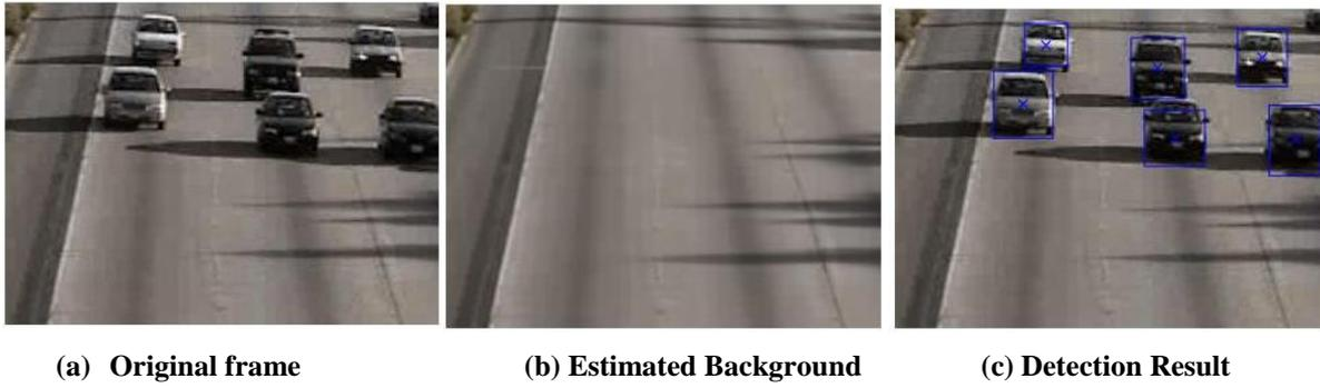
Figure 6: Frame No. 140 Complete Result
