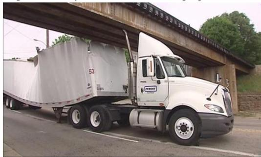
**Figure 1. The laterally impact load with bridge girders**
