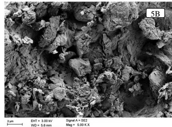
Figure 5 Micrograph of untreated soil (5A) and treated soil (5B) under magnification of 5.00 KX
