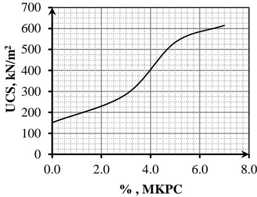
Figure 3: unconfined compressive strength results
