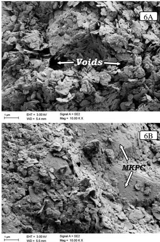
**Figure 6: Micrograph of untreated soil (6A) and treated soil (6B) under magnification of 10 00 K X**
