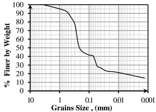
**Figure 1: Grain size distribution for the test soil**
