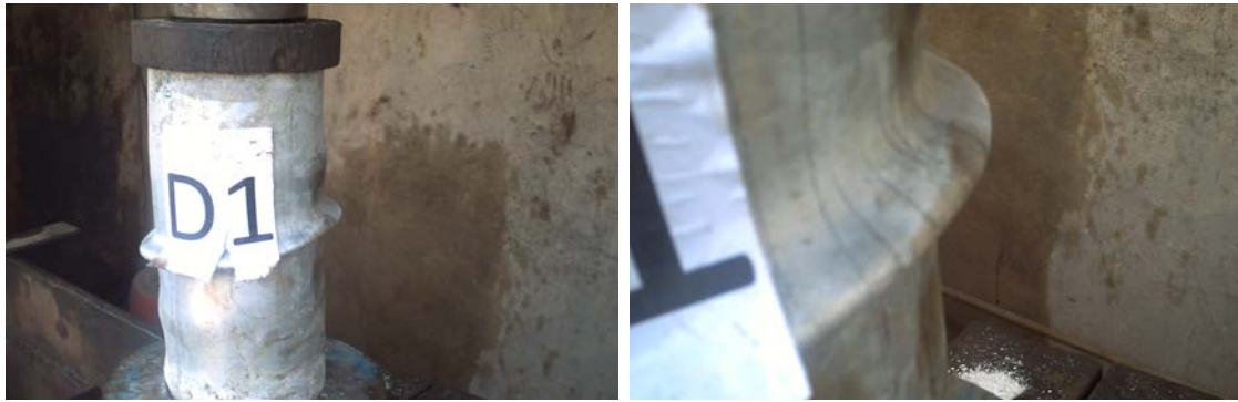
Fig. (17): Failure Pattern of Sample D1
