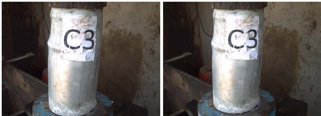
Fig. (15): Failure Pattern of Sample C3
