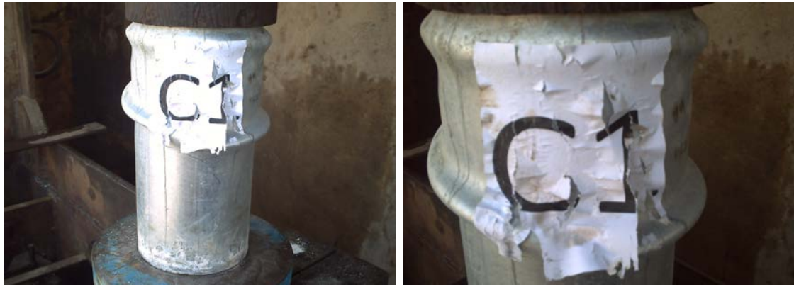
Fig. (13): Failure Pattern of Sample C1
