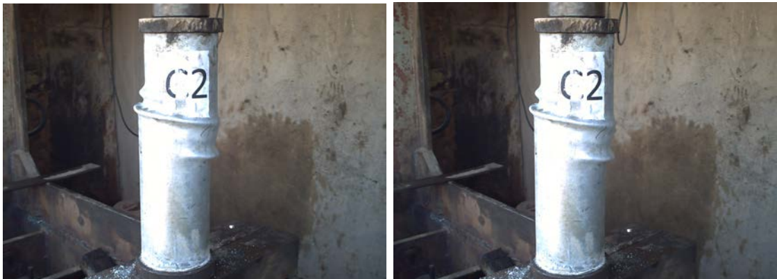
Fig. (14): Failure Pattern of Sample C2
