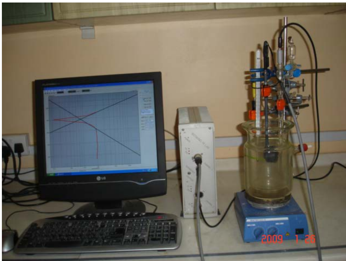
Fig (2): A photograph of the electrochemical corrosion unit
