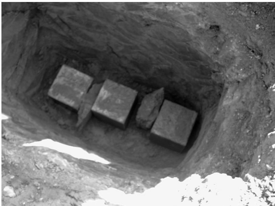
Plate (4) shows putting samples and backfilling hole in zone B
