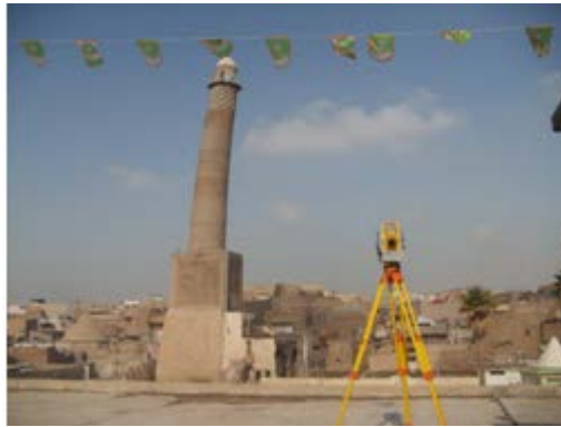
Figure 2. Topcon Imaging Station at monitoring work.
