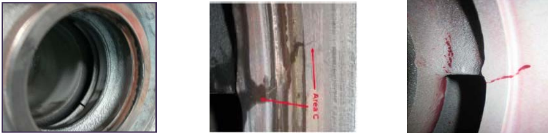
Figure (1-1) Shows failure via thermal cracking[2]
