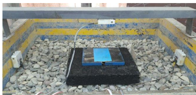
Figure 4. Pavement layers in unreinforced model.
