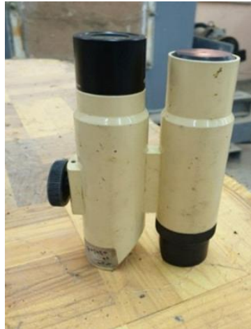
Figure 5. Crack meter device.
