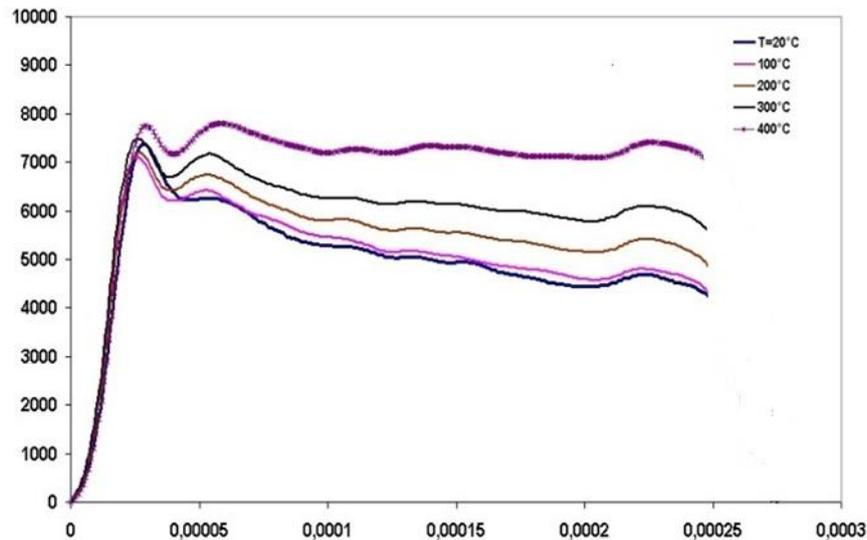
**Fig. 3:** Experimental speeds applied to the interface of the simplified model for various temperatures at impact velocity 11.5 m/s of aluminum copper alloys
