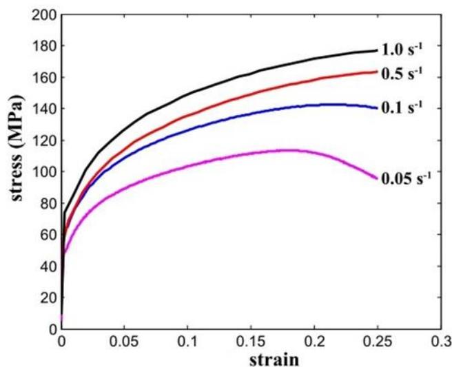
**Fig. 4:** stress-strain curves of aluminum copper alloys
