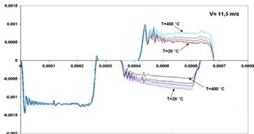
**Fig. 2:** Experimental signals of the elastic deformation in the bar incident at various temperatures at the impact velocity of 11.5 m/s
