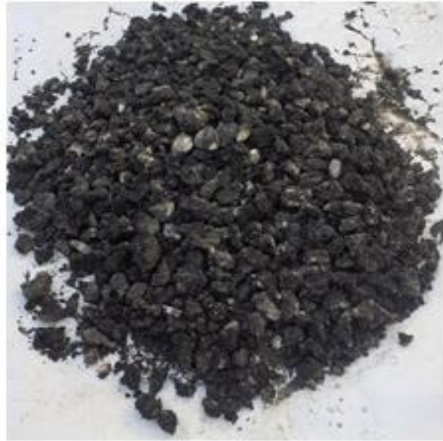
Fig. 2: Crumble old pavement
