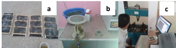
Plate 1: experimental setup: (a) specimen preparation, (b) flow and (c) flexural testing apparatus in the University of Technology.
