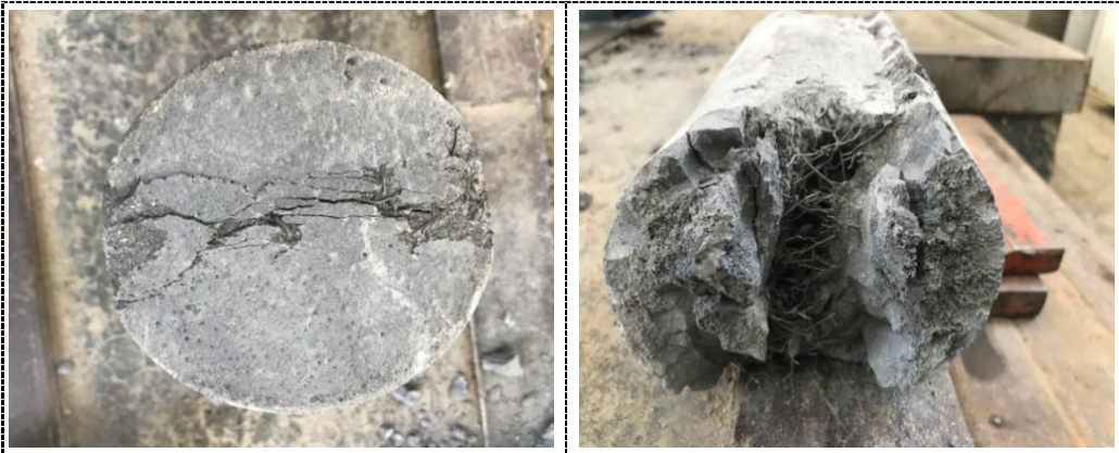
Fig. 9: Splitting tensile crack patterns
