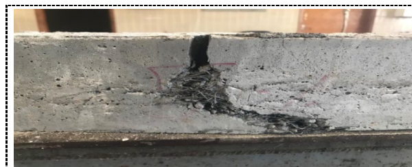
Fig. 11: Prism failure patterns
