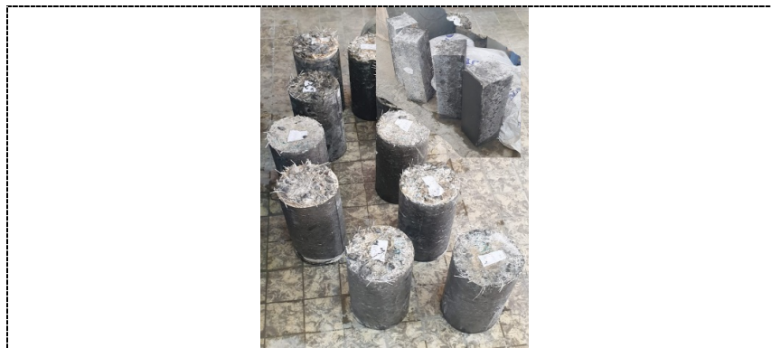
Fig. 3: Compressive, splitting and flexural specimen's test.
