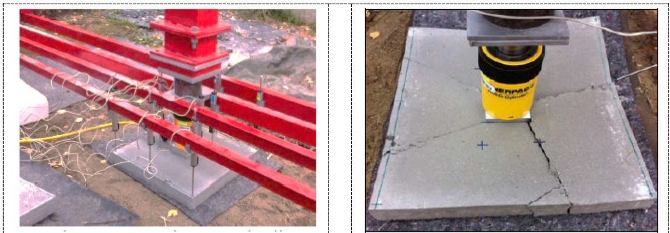
Fig. 1: Testing view and failure model.
