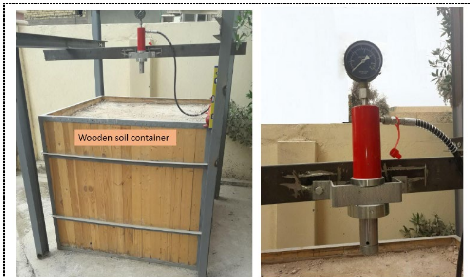
Fig. 5: Hydraulic jack hanging.
