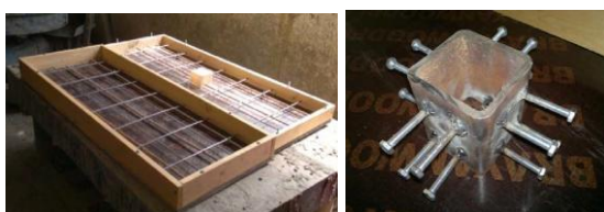
Fig. 7: Specimens and steel plate used for strengthening [9]
