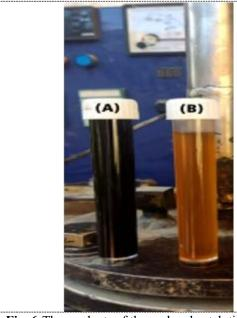
Fig. 6: The products of thermal and catalytic cracking process of RCR at the optimum operational conditions.
