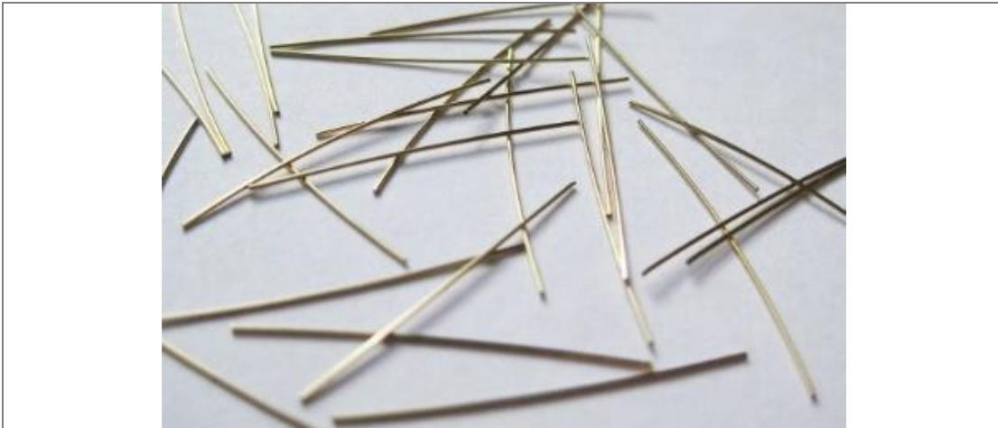
Fig. 5: Straight steel fiber used by Yang et al. [46]
