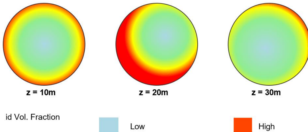
Fig. 6: Contour plots of instantaneous solid volume fraction at different riser heights ( z=10\text{m} , 20\text{m} , and 30\text{m} ), illustrating the development of the core-annulus flow structure
