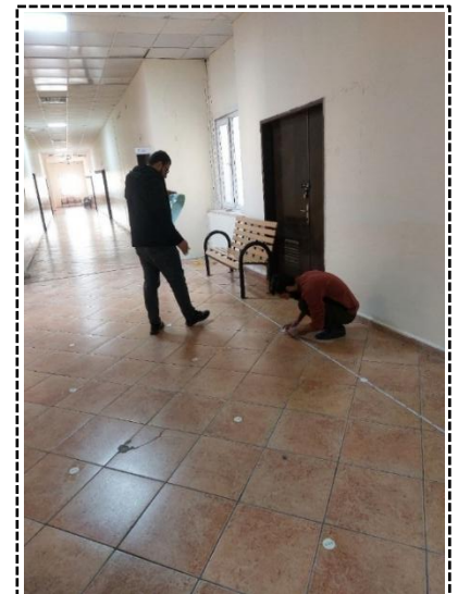
Fig. 3: Reference point deployment showing grid spacing measurement (1.02 m intervals) and coordinate verification from fixed architectural landmarks.
